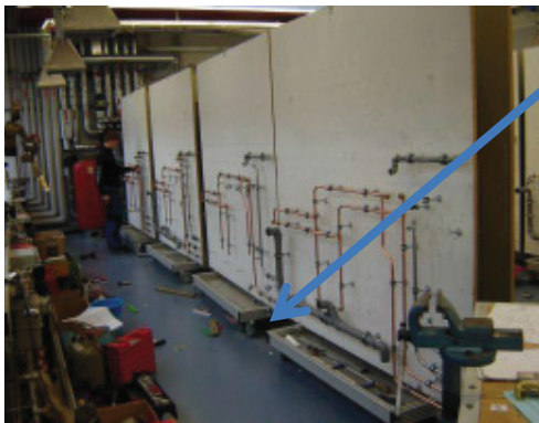
Mobile work units for plumbers in Germany,(*1)
