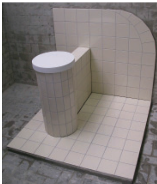
Removable test setting for tilers *6
