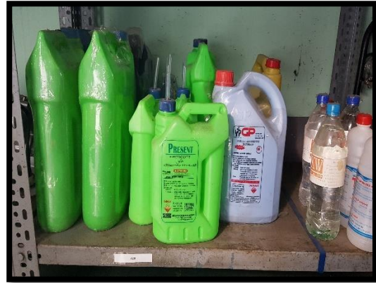
Hazardous material not proper stored in a structured way
